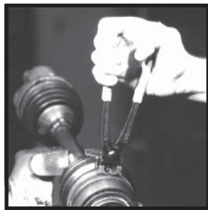
Cartridge Roll & Arbor Assembly: For Polishing Ball Wear in Joints
