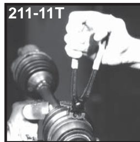
211-11T Banding Tool: For Crimp Type Clamps
